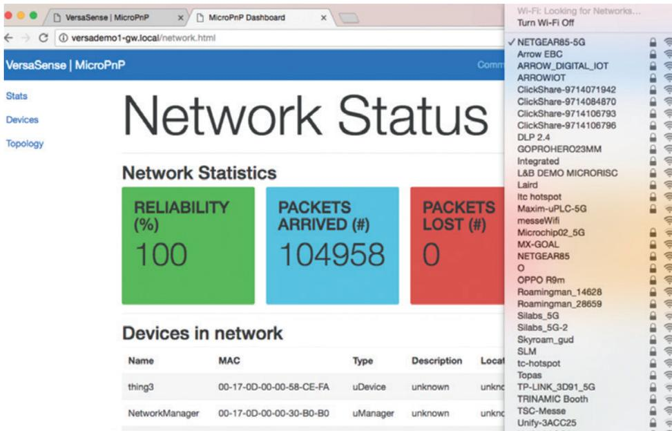
**Figure 2. Network Reliability at Electronica 2016—Even in the Presence of Over 50 Wi-Fi Networks, the SmartMesh IP Network Delivered Over 75.5Mbits of Data (104,958 Packets of 90-Byte Payload) at 100% Data Reliability**
