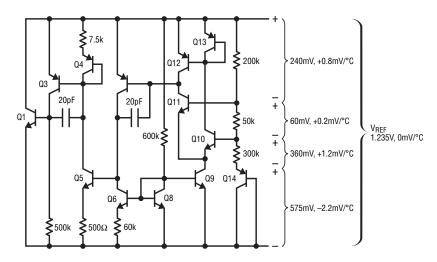
Figure 5. A bandgap circuit is designed for a theoretically zero temperature coefficient.
