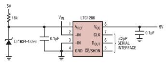
Figure 1. Typical use of a voltage reference for an ADC
