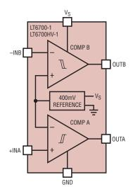
Figure 7. The LT6700 allows comparisons with thresholds as low as 400mV.
