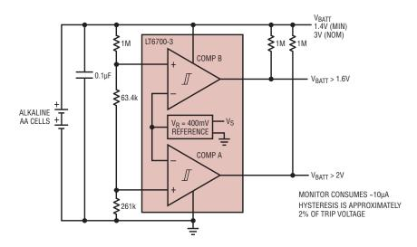
Figure 8. Higher thresholds are set by dividing the input voltage.
