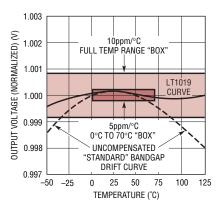
Figure 2. Voltage reference temperature characteristics
