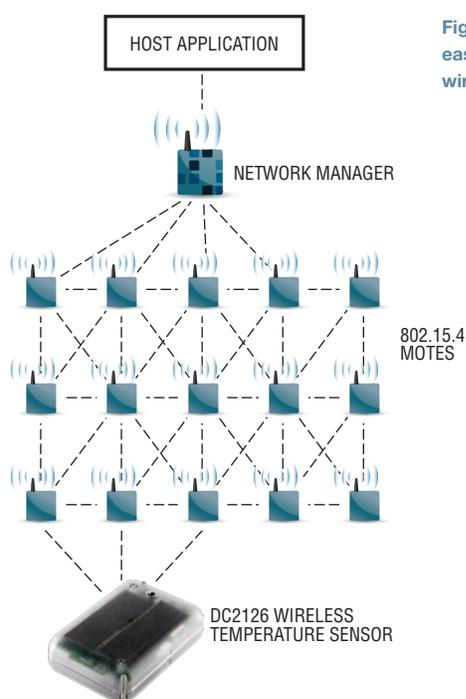
Figure 6. Precision temperature sensor easily drops into robust SmartMesh IP wireless mesh network.
