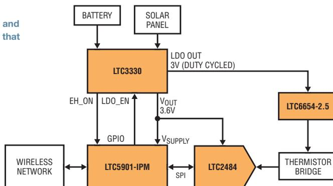
More sensors means better plant monitoring. The achievable number of industrial sensors can be multiplied by eliminating all cabling requirements through the use of robust, wireless, micropower sensors that run for years on a small battery. Better yet, eliminate the need to replace or recharge batteries. Instead, sensors harvest energy from their immediate environment, taking advantage of locally available energy sources, such as light, vibration or temperature gradients.
