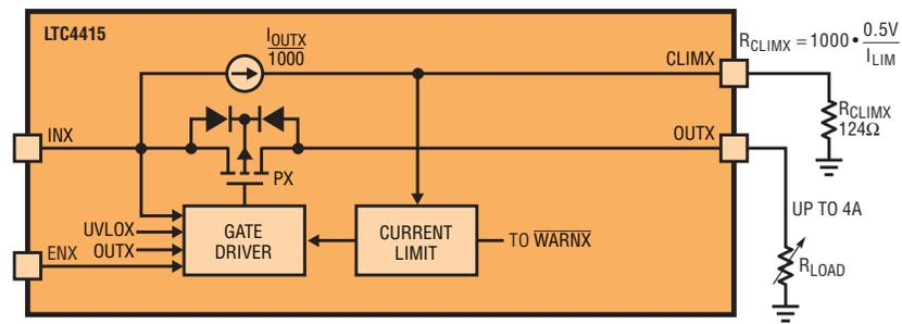
Figure 4. Current limit detection inside the LTC4415 for each channel
