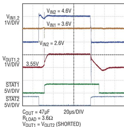
Figure 5. Rapid path switchover with only 5% transient voltage dip
