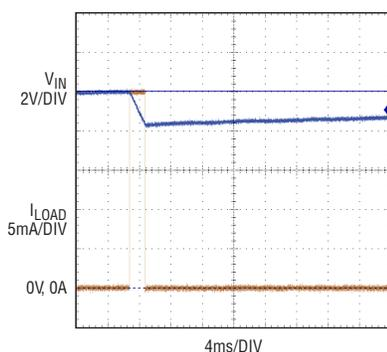
Figure 2. Charging with sensor-transmitter load
