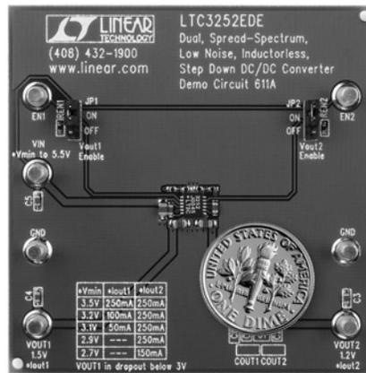
Figure 1. A complete dual output Li-Ion converter
