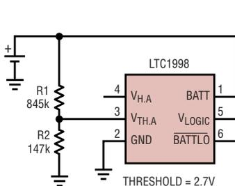
Figure 1. Threshold adjustment with resistor divider
