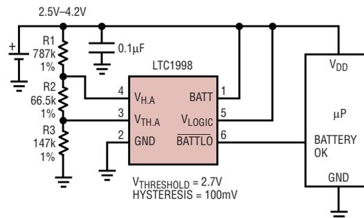
Figure 2. Single resistor divider sets both thresholds
