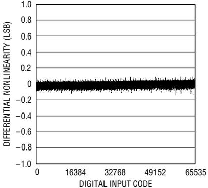
**Figure 3b. DNL for Figure 1's circuit**
