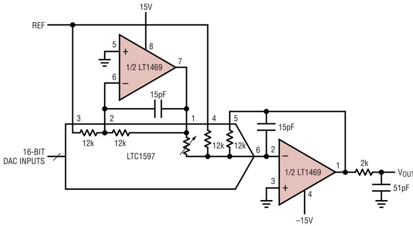
**Figure 1. 16-bit DAC I/V converter and reference inverter**
