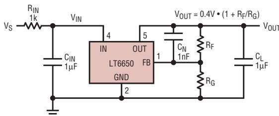
Figure 4. Simple input network for improved supply rejection
