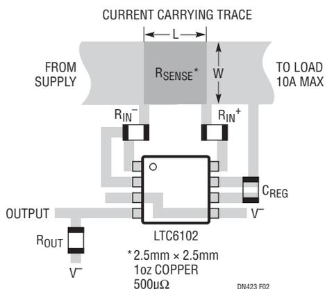
Figure 2. LTC6102 Layout Using Printed Sense Resistance
