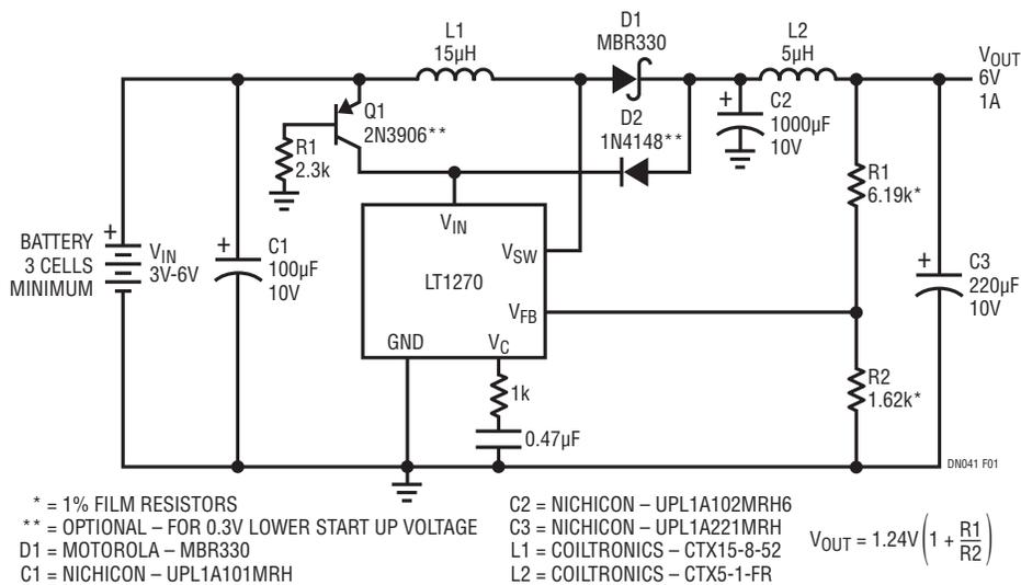
Figure 1. Low Voltage Circuit Provides Constant Output Voltage as Battery Discharges
