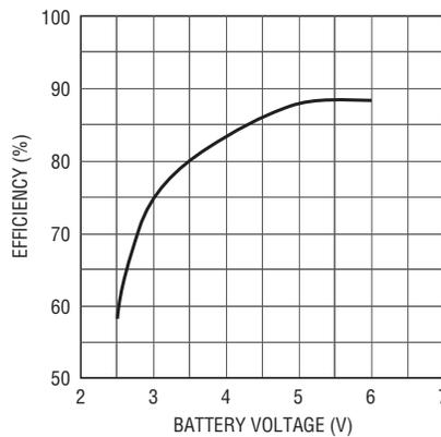
**Figure 4. Efficiency for Various Battery Voltages**
