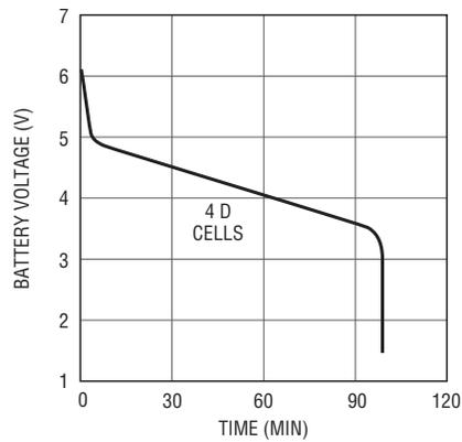
**Figure 3. Alkaline Battery Discharge Characteristic with 6W Load**
