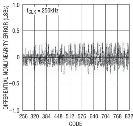
**Figure 2a. Differential Nonlinearity, Power Supply Voltage Mode**
