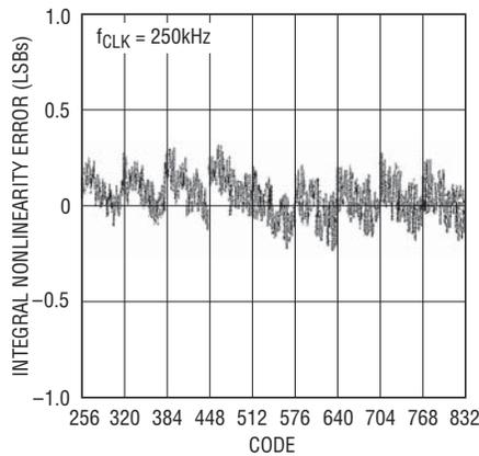
**Figure 2b. Integral Nonlinearity, Power Supply Voltage Mode**
