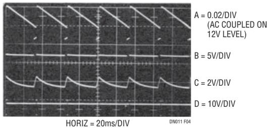
Figure 4. Waveforms at 3mA Load for Figure 2
