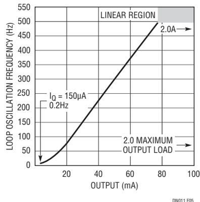
Figure 5. Output Current vs Loop Oscillation Frequency for Figure 2
