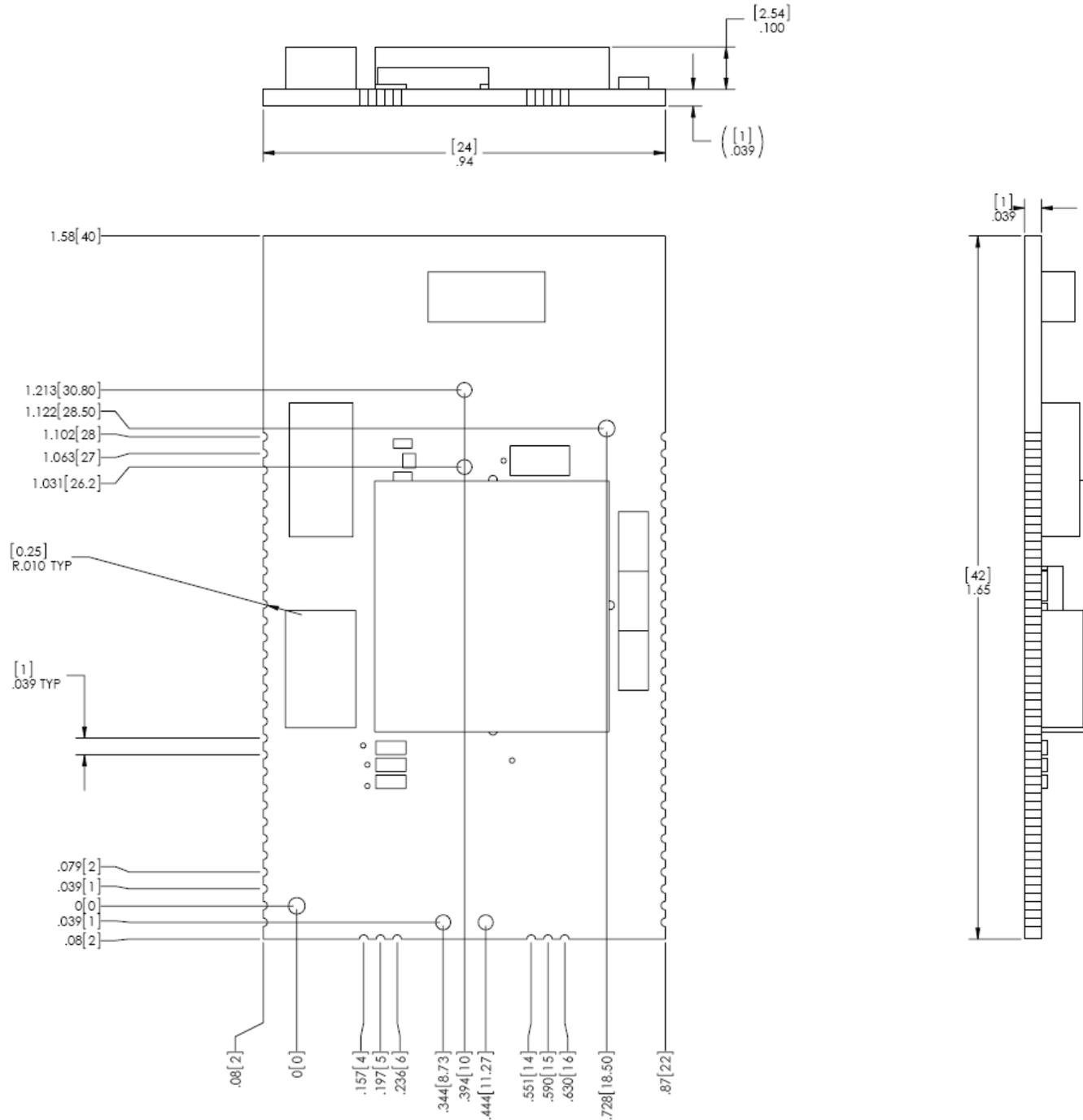
Figure 3 Mechanical Drawing – LTP5901
