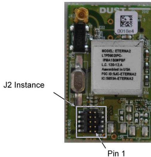
J2 per the pinout shown below, provides both power and connection to ETERNA2's CLI port. Connection to pins 1 through 6 are optional for CLI access.
