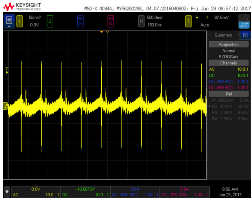
Figure 4. DC2598A, LT8390A Output Ripple Measured at C45
