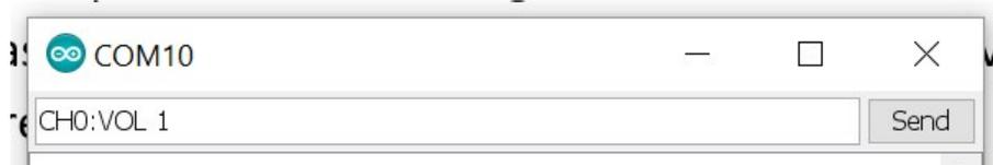
The terminal responds with the voltage value that has been set, and the voltage on the output changes. In this case, CH0's output will be configured to 1.0000V.
