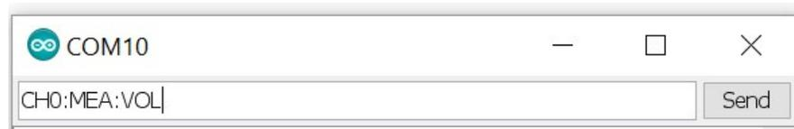
On this EasySMU, the response is 0.9977. The voltage measurement is more accurate than the setting value, so it can be concluded that the output voltage is 0.9977V.
