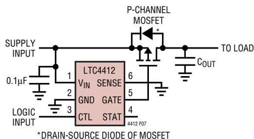
**Figure 7. Logic Controlled High Side Power Switch**
