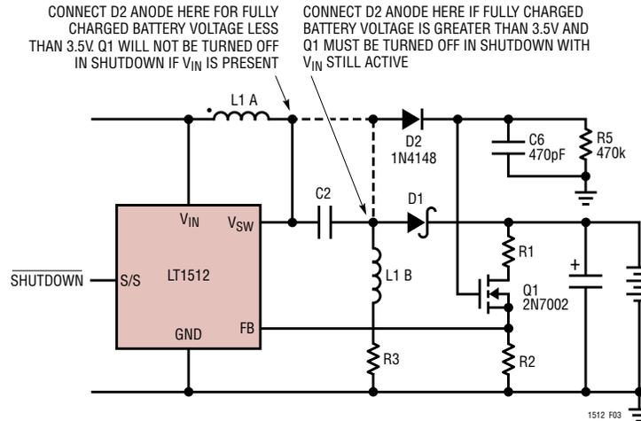
Figure 3. Eliminating Divider Current
