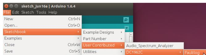
**Figure 2. Loading Fault Log Sketch**
